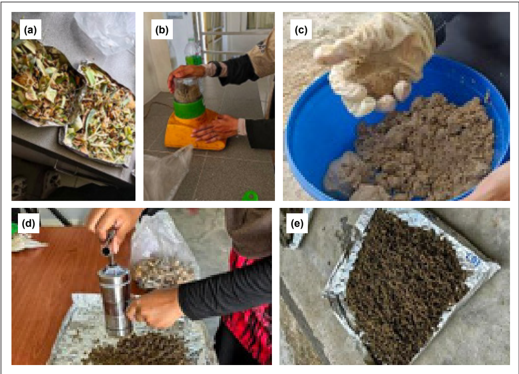
Figure 1. Utilisation of pineapple waste for pellet production: (a) Pineapple waste was collected for the drying process; (b) After drying process, the pineapple waste was ground by using a blender; (c) Mixed all the ingredients, mix it up and shape it into a circle; (d) Put it in the grinder to form pellets; and (e) Dry it out under the sunlight and in the oven (70-100 °C)
